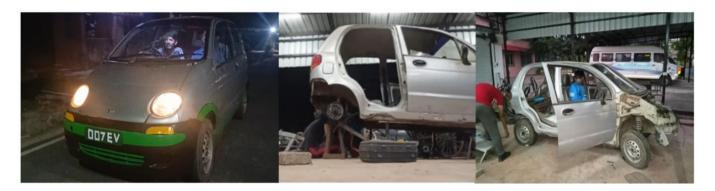
We successfully transformed a Daewoo Matiz Scrap car into an electric vehicle, leveraging its front-wheeldrive system by placing the electric motor and differential to the rear. Powered by a series of twelve 72V lead-acid batteries, our innovative conversion delivers a substantial 50km range. This project not only breathes new life into a retired vehicle but also showcases our commitment to sustainable and eco-friendly transportation solutions.
