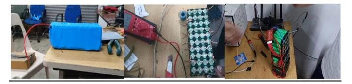
Our recent accomplishment involves the meticulous assembly of a Li-ion battery pack utilizing highquality 18650 cells, each rated at 3.7V. Through careful design of dimensions and connections, we've successfully crafted a powerhouse that outputs 36V with a substantial 10Ah capacity. What sets our creation apart is the inclusion of a sophisticated Battery Management System (BMS), ensuring not only optimal performance but also precise charge balancing for enhanced longevity and reliability.
